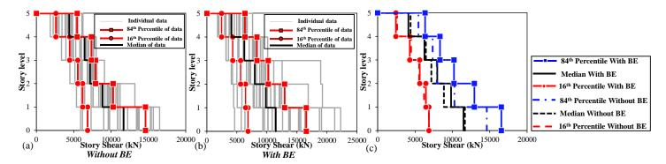
Figure 7. Response Story Shear Variation before and after Boundary Elements: (a) Without Boundary Elements; (b) With Boundary Elements; (c) Comparison prior and after adding Boundary Elements.
