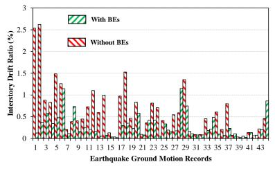
Figure 8. Inter-Story Drift Variation of the RMSW Building before and after having Boundary Elements
