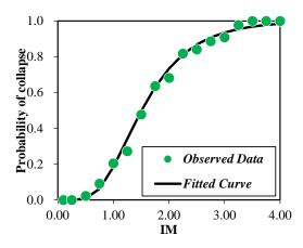
Figure 5. Sample Fragility Function Curve Fitting
