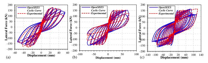
Figure 2. Comparison of Numerical versus Experimental Hysteretic loops: (a) W1; (b) W2; and (c) W3 (Experimental data from Shedid et al. 2010)
