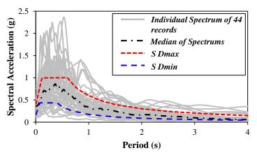
Figure 3 Response Spectrum of 44 unscaled Ground motions along median spectrum; Upper bound (S Dmax); and Lower bound (S Dmin)
